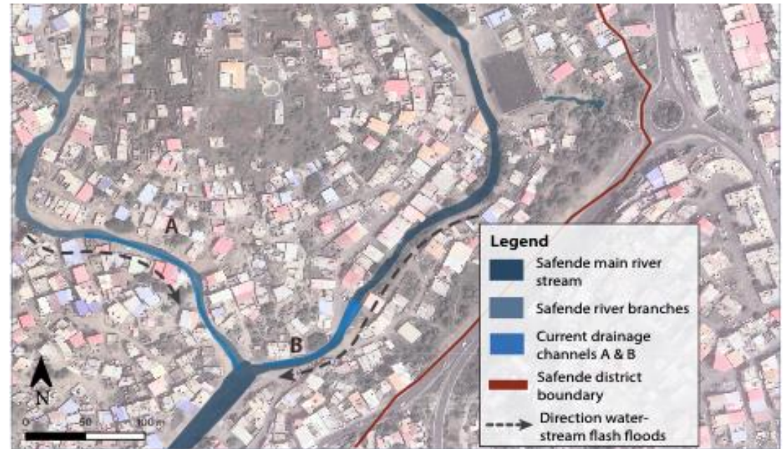
Figure 14 Drainage channels built in 2019 (Source: A. Sayyad-Hartounian).
